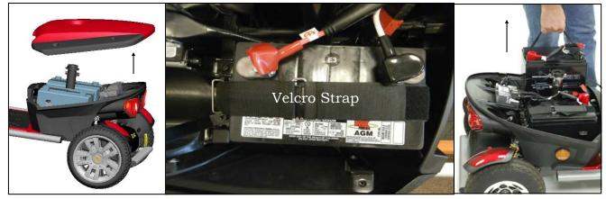
Figure 12. Removing the Batteries
