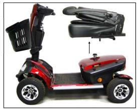
Figure 11. Removing the Seat
