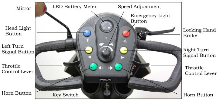
Figure 5. Patriot<sup>TM</sup> Delta Tiller Control Panel
